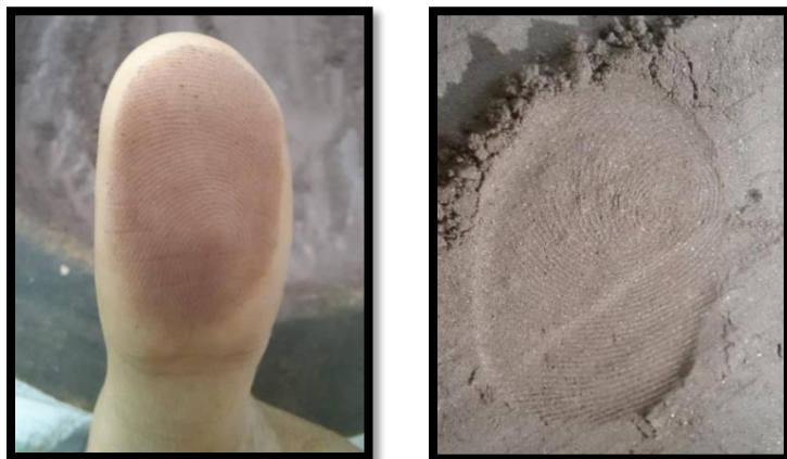
Fig 01: KC impinged in the furrow of finger (Fingerprint test)
